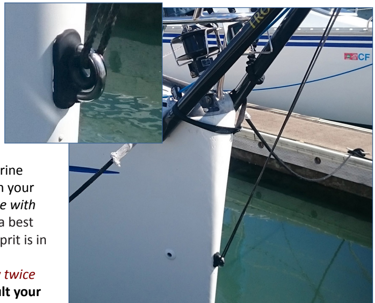
Fig 11: U Bolt attached to the bow.
