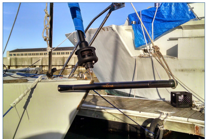
Fig 12: Temporarily secure the Bowsprit with a line
